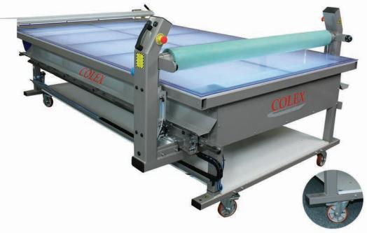
The pressure roller has 5/8" thick soft rubber coating to guarantee the bubble free & crease free application. The pressure roller is controllable from both sides. The pressure of the roller can be adjusted within a wide range by the pneumatic controllers. The castors with brakes allow the table to be easily moved or fixed in position.
