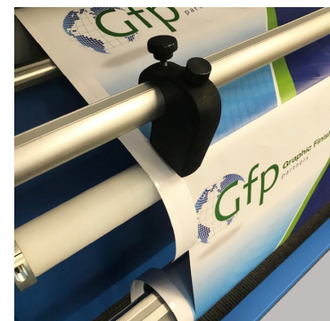
INLINE ROTARY SLITTERS trim the sides of output during lamination to save time and increase productivity.
